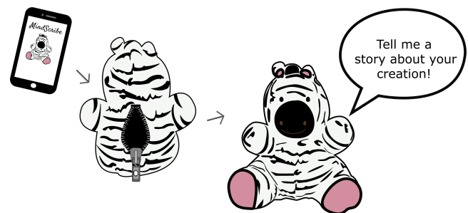
Figure 2: A graphic of our initial child-robot interaction. A mobile application running the voice interaction is inserted into a stuffed animal (stuffedie) embodiment. We instruct the children, “We put the phone in the stuffedie, to make the stuffedie talk.”
